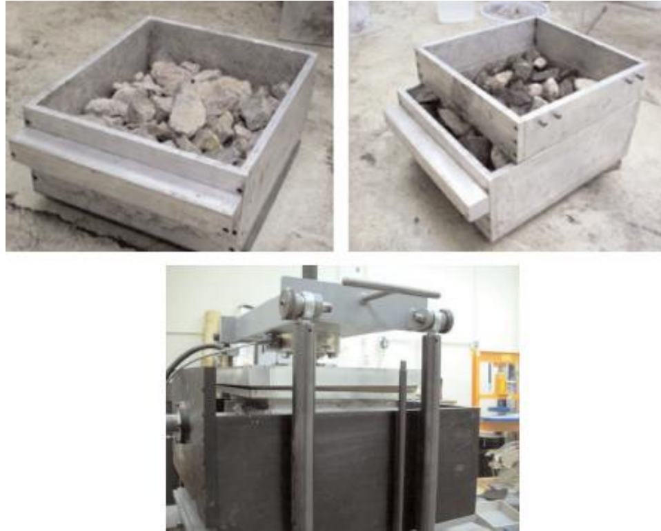
Figure 3.9 Photograph of Direct Shear Test Equipment at the University of Illinois at Urbana-Champaign (Huang et al., 2009)
